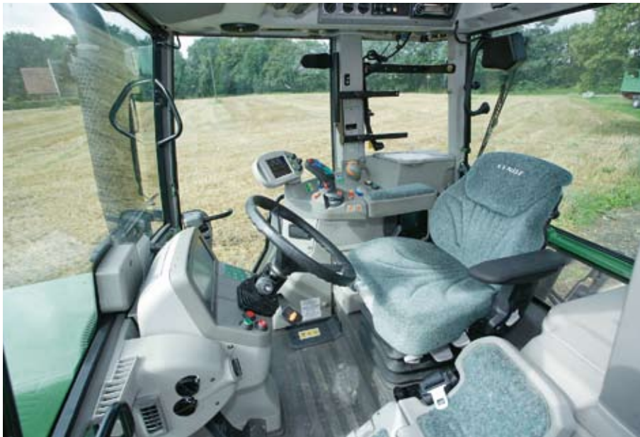
Air conditioning, yes; climate control, no. And space within the Fendt 820 cab is at a premium, too. Countering this, the accommodation is pleasantly quiet at 72.3dB(A). Photos: ST.
