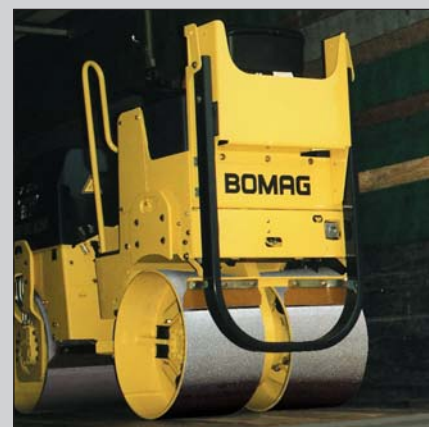
The folding ROPS make transport easier
