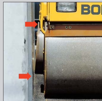
BW 80 ADS up against the wall: No damage, no follow-up working
